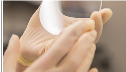
The aberration-corrected multi-focus microscopy (MFM) technology developed by Abrahamsson requires custom-made diffractive gratings. (Photo by Carolyn Lagattuta)
