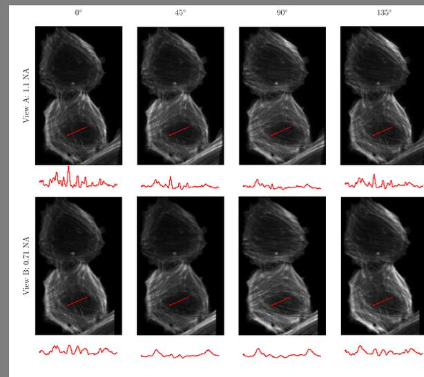
It captures four polarization-sensitive stacks from each of two orthogonal directions.
