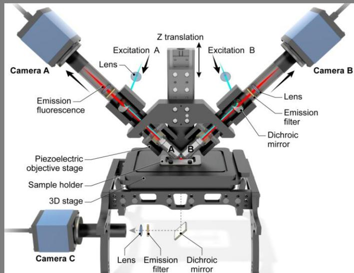
We have added polarization filters to the excitation channels of a diSPIM dual-view light-sheet microscope
