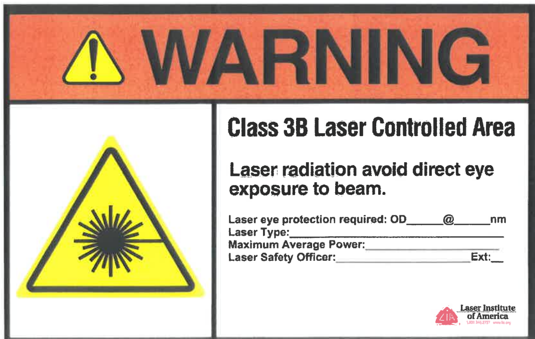
Figure 2. Sample warning sign for certain Class 3R, Class 3B, and Class 4 Laser Controlled Areas. Adapted from ANSI Z36.1-2014 (Figure 1b).
