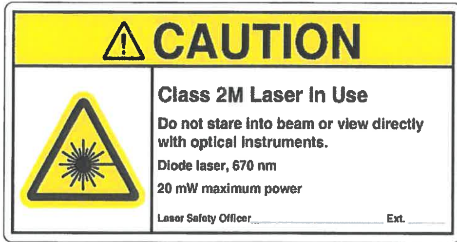
Figure 1. Sample warning sign for Class 2, Class 2M, and Class 3R lasers. From ANSI Z36.1-2014 (Figure 1a).
