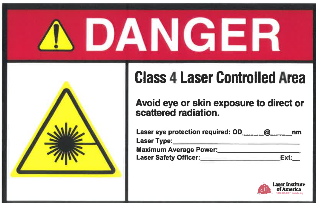
Figure 4. Sample warning sign for Class 4 Laser Controlled Area. Adapted from ANSI Z36.1-2014 (Figure 1c).
